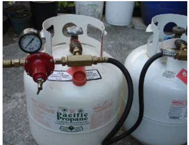
Hoses, regulator, gauge and connectors.
