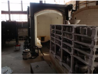
The Iwashita kerosene-fired car kiln, stacked and ready for loading.
