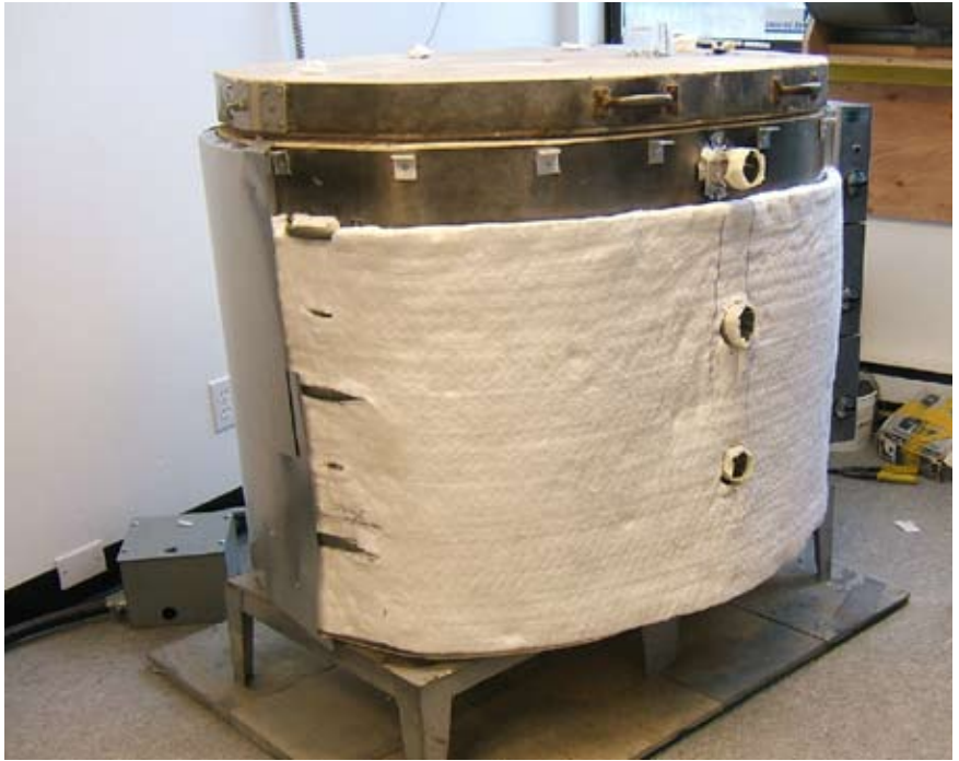
Wrapping the front of the "free" kiln.
