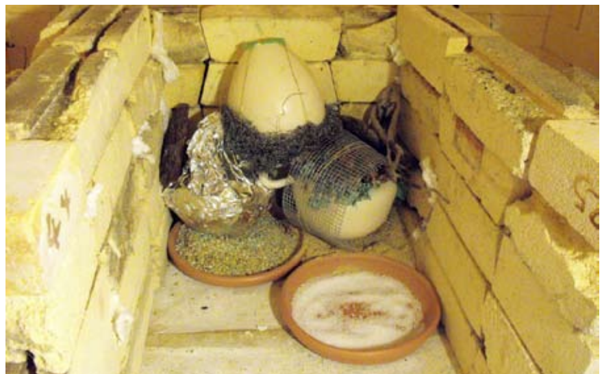
Three walls of the saggar are completed. Wrapped ware and combustible materials are tumble stacked.
