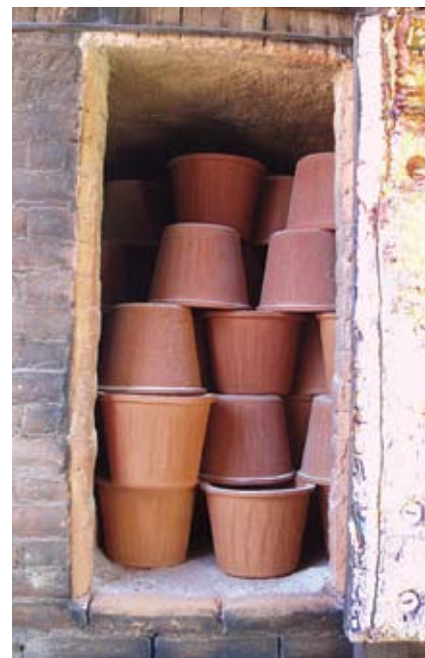
Fired filters ready to be unloaded from the kiln.
