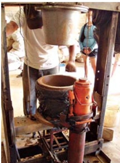
Mould is raised out of the pressed clay filter.
